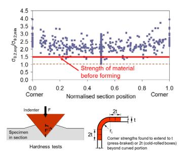
Mechanically based predictive models developed and verified against collated tests; two-step process:
