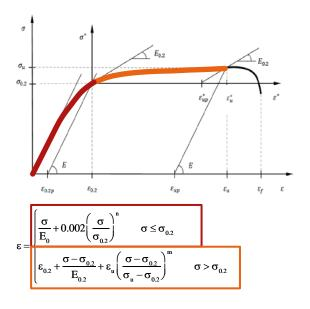
Equations based on austenitic and duplex grades. Not always valid for ferritics. A revision is needed to represent all grades.
