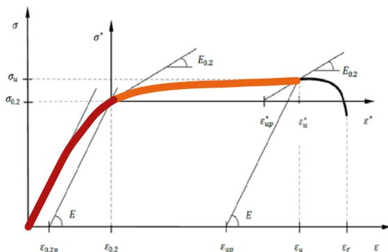
$$\epsilon = \begin{cases} \frac{\sigma}{E_0} + 0.002 \left( \frac{\sigma}{\sigma_{0.2}} \right)^n & \sigma \leq \sigma_{0.2} \\ \epsilon_{0.2} + \frac{\sigma - \sigma_{0.2}}{E_{0.2}} + \epsilon_u \left( \frac{\sigma - \sigma_{0.2}}{\sigma_u - \sigma_{0.2}} \right)^m & \sigma > \sigma_{0.2} \end{cases}$$
