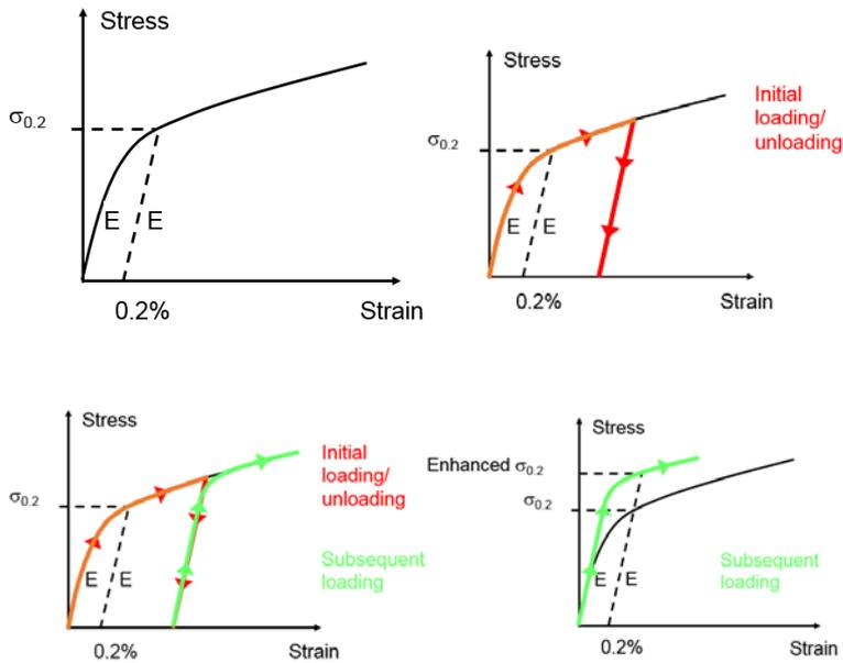
37 By slicing specimens into a series of strips and then measuring the stress-strain characteristics it is possible to build up a profile of strength around the section. With sufficient data, predictive tools can be developed – this process is underway at the moment.
