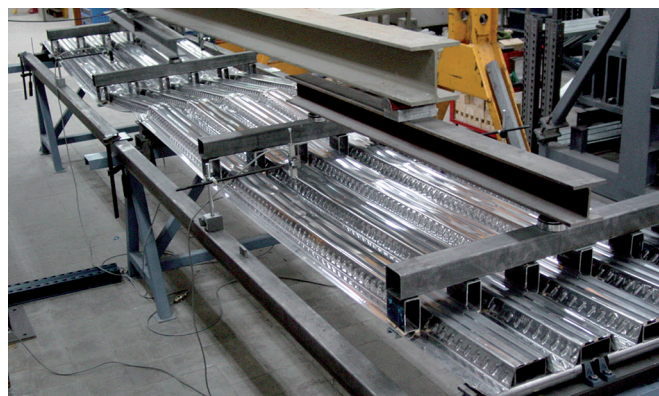
Figure 9 Continuous decking tests at the construction stage
