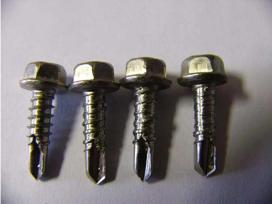
Figure 5: Austenitic stainless steel self drilling crews, too soft to cut the thread.
