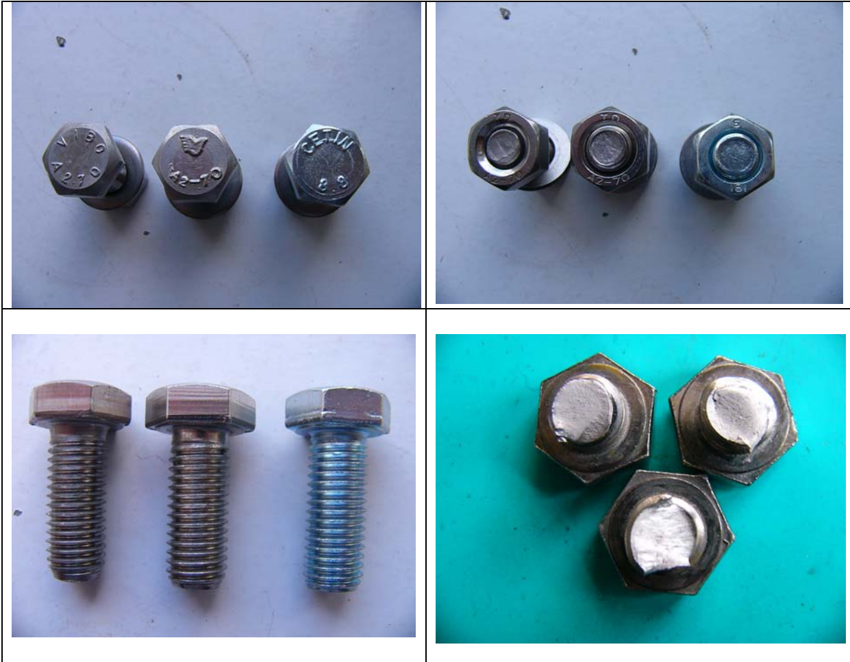
Figure 4. Bolts and nuts applied in tests and destroyed bolts
