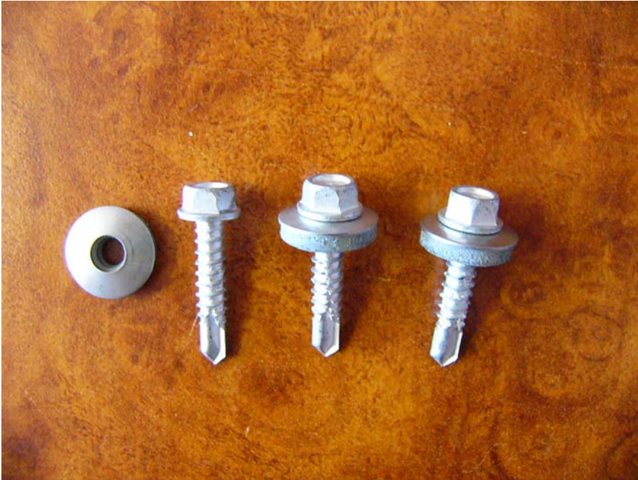
Figure 6: Self drilling screw A2TiIV, 5.5 x 25 mm, DIN 7504-K/POR, able to cut the thread into predrilled hole.
