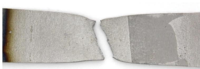
**Fig 35. A ductile base metal fracture in autogenous TIG weldment of 1.4509.**
