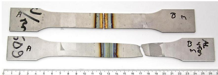
**Fig 62. Tension test samples, both originally 235 mm in length. Notice the brittle fracture in 1.4016 (top) without any elongation. A more ductile fracture has occurred with 1.4509 from the base metal (bottom).**
