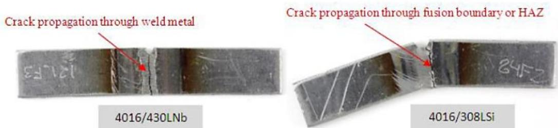
**Fig 43. Crack propagation in the weld metal impact toughness test. Welds fabricated with ferritic 430Nb (left) and austenitic 308LSi filler metals (right). The latter weld cracked through the HAZ, even though the notch is located at the centre of the weld.**
