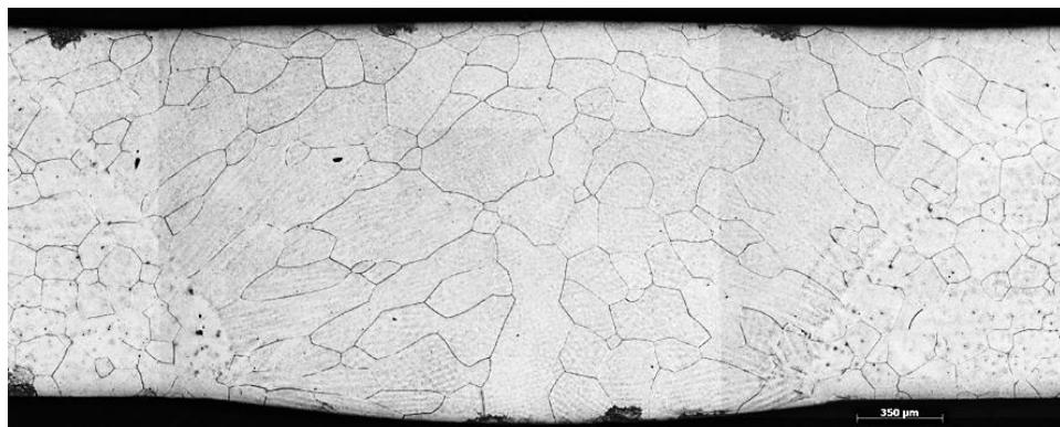
**Fig 33. Autogenous TIG weld metal of grade 1.4621, 1.5 mm thickness, heat input 0.16 kJ/mm, welding speed 106 mm/min. Large-grained weld metal.**
