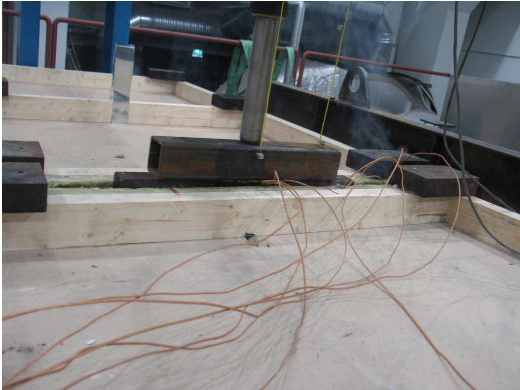
Figure 5. Unexposed face of test specimen 1 at the test time 15 min 51 s.
