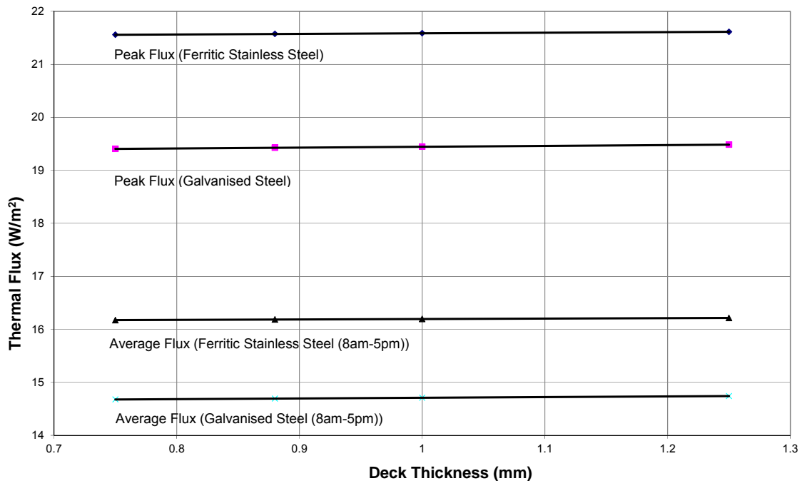
Figure 3-3 Thermal flux ( W/m^2 ) on bottom surface per horizontal metre for galvanised steel and ferritic stainless steel deck for various deck thicknesses.
