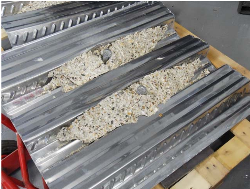
Figure 16 Failed specimen – decking
