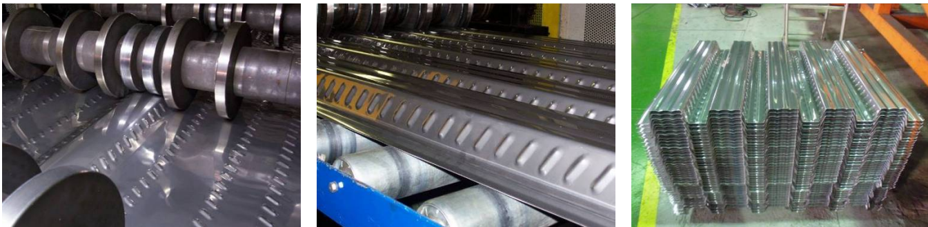
Figure A-2 : Roll-forming trials of Cofraplus 60 decking
