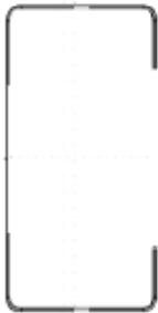
Figure 1: Effective section of Lipped channel 36.0x72.0x15.0 1.0 mm
