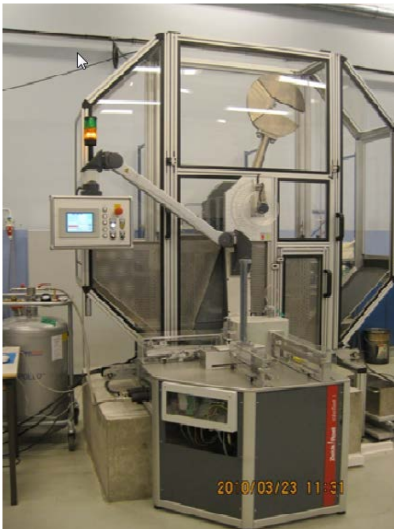
Figure 2 Instrumented Zwick Roell PSW 750 impact tester.
