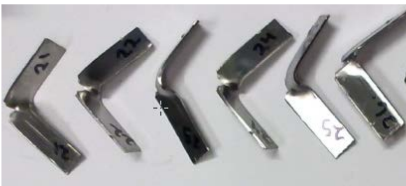
Figure 4 Twisted specimens with a thickness of 1 mm.
