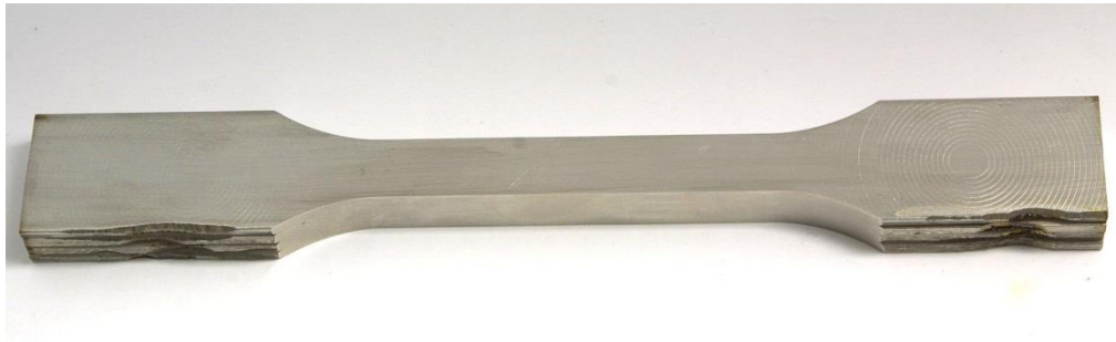
Figure 3. Laminated test piece used for compression testing.
