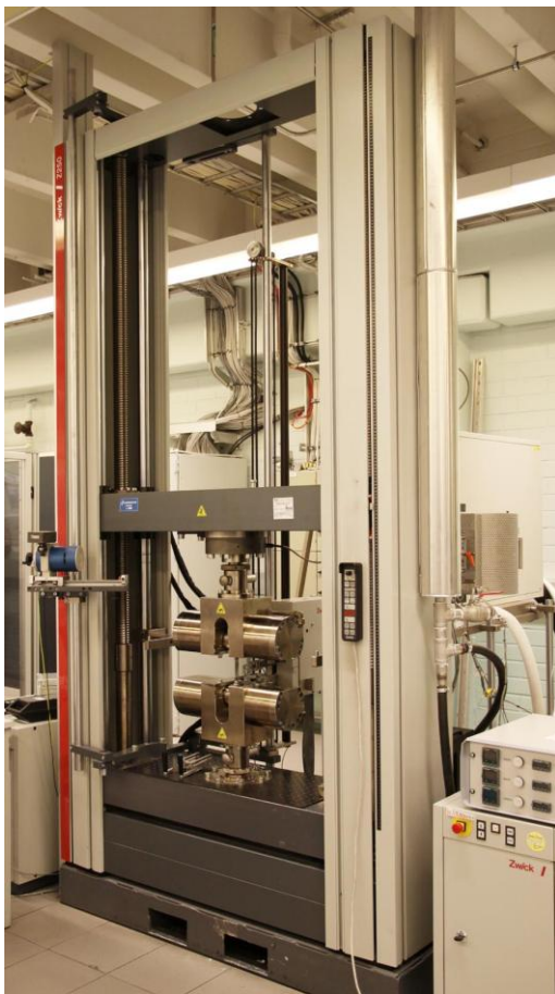
Figure 1. Zwick / Roell Z250 tensile test machine used.
